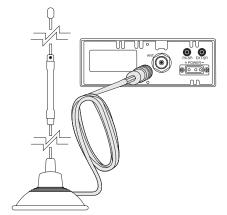
Connect the antenna cable plug to the receptacle marked "ANT" on the back of the unit.
