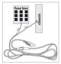
**4.** Connect the red lead of the DC power cord to an accessory 12 volt fuse or directly to the battery.
