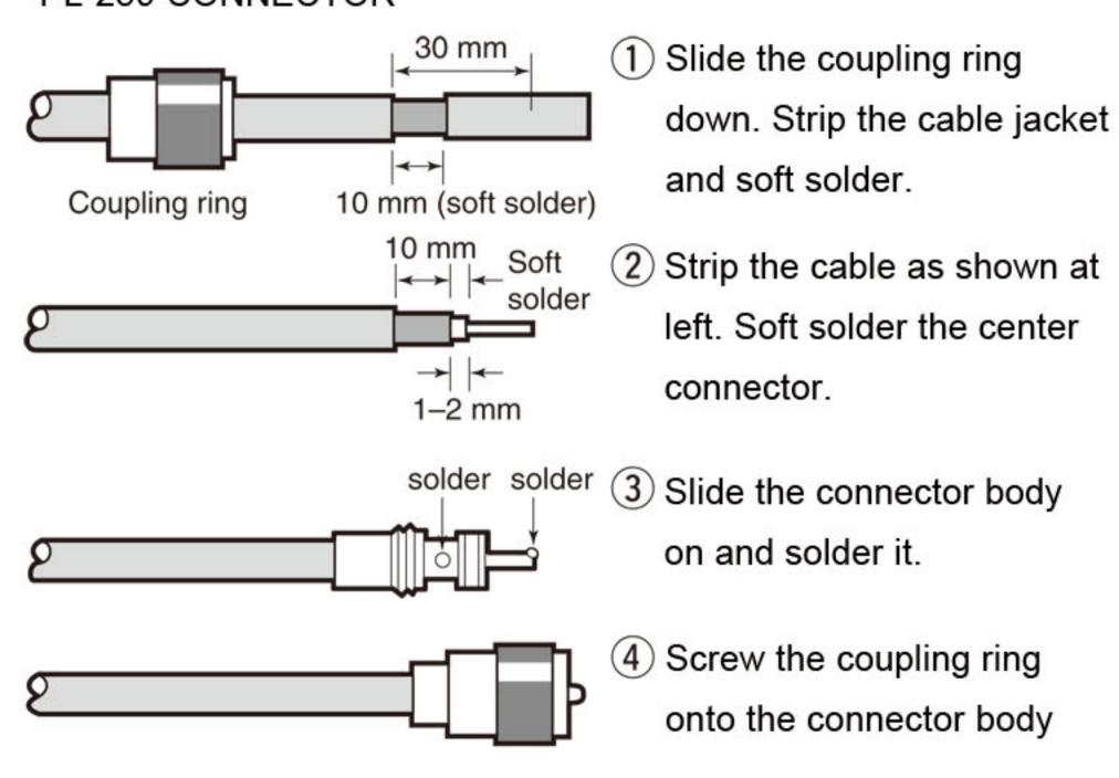
**NOTE:** There are many publications convering proper antennas and their installation. Check with your local dealer for more information and recommendations. Connects a  $50\Omega$  antenna with a PL-259 connector and a  $50\Omega$  coaxial cable.
