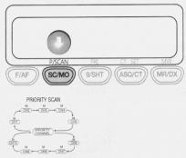
With Priority Scan function the Radio scans for activity, but in addition, it also inserts your Priority Channel into the scan sequence.
