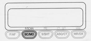
Venus CB transceiver incorporates a scanning feature. The radio will scan through all 40 (80) channels and will stop at BUSY channel. The default stay time is 5 seconds after conversation has stopped and then it will resume scanning.
