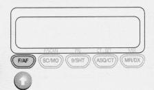
You can select AM or FM modulation by pressing the F/AF button for 2 seconds. Please note that in the German 80 CH system it is possible (and allowed) to listen in AM on all 80 channels but transmit is only possible on CH 1 - 40 in AM. During receive mode, The bar graph shows the strengths of the received signal, during transmission, it shows the relative output power.
